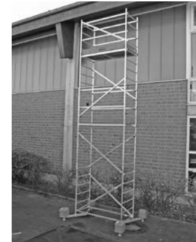
Basic scaffold with first and second extension
